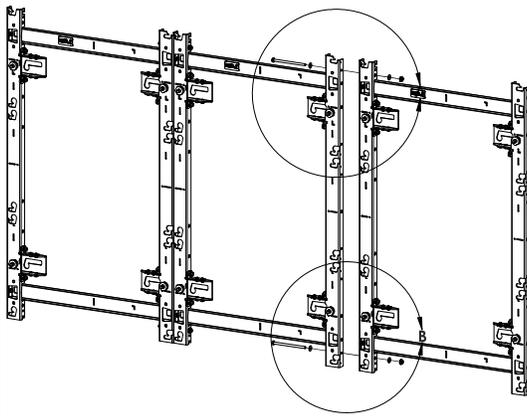
MOUNT SECTIONS ARE CONNECTED USING 1/4-20 BOLTS, INCLUDED. ONE SIDE HAS HOLES AND THE OTHER IS SLIGHTLY SLOTTED TO ALLOW FOR ANY ADJUSTMENT PRIOR TO TIGHTENING AND CLAMPING THE MOUNTS TOGETHER.
